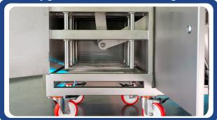
All electrical components are safely positioned above floor level, keeping the underside clear for full washdown access. This open, elevated design reduces contamination risk and supports rigorous hygiene compliance in food production environments.
